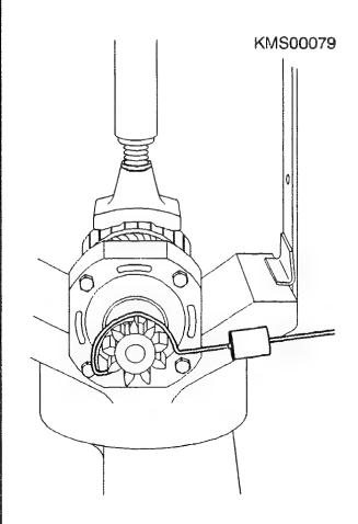
CHECKING AND REPAIRING COMPONENTS Checking multi-plate clutch Check clutch overload protection. Slip support sleeve over drive spindle into intermdiate bearing and insert pinion in drive spindle. Use torquemeter to check response torque in friction direction. Torquemeter: 0 986 617 166 Support sleeve: 0 986 617 164 Response torque, overload
